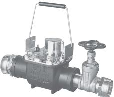
The Fire Hydrant water meter is designed for mobile use in metering flows from fire hydrants. The meter measures a wide flow range to maximize revenue. It meets or exceeds the latest performance requirements of AWWA. Maximum flow rates may be exceeded by 25% for intermittent flows.
